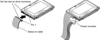
**Note.** If your computer does not have an unused power cable for your new hard drive, you can purchase a Y-shaped power splitting cable from your computer dealer which effectively converts one power connector into two.
